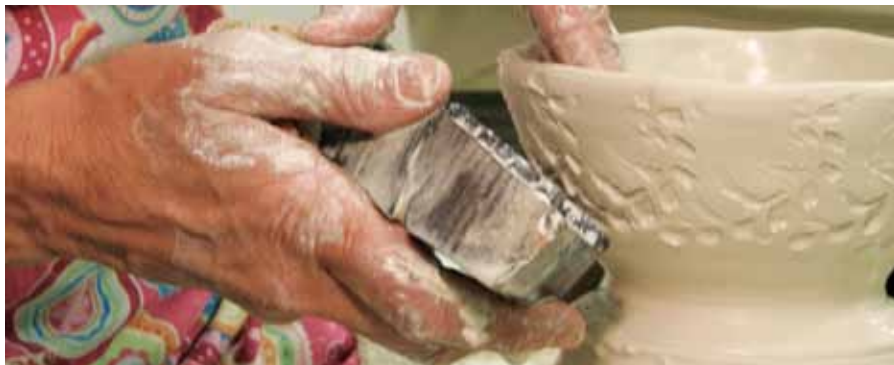
Wooden textile-printing blocks are wetted to prevent them from sticking to the clay. They are pressed into the surface while the form, thrown slightly thicker than normal so it can stand up to the stamping, is supported from the inside.
